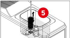
• Place a bucket under the dispensing door, activate the beater rotation and release the rinse water.
