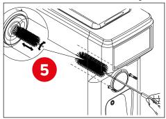
• Soak the brush in the sanitizing solution and clean the cylinder.
