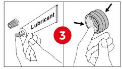
Lubricate and install the beater seal.
