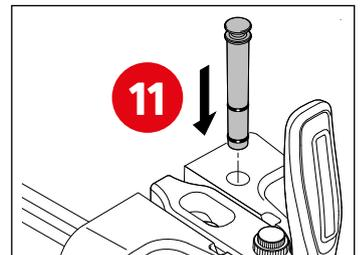
Install the 2 O-rings on the prime tube, lubricate and install it in its seat on the dispensing door.
