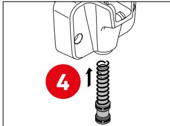
Place the spring on the piston, install the piston in its seat on the dispensing door and match it with the handle pin.
