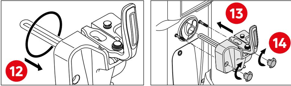
Insert the seal in place, fit the dispensing door and secure the fastening knobs.
