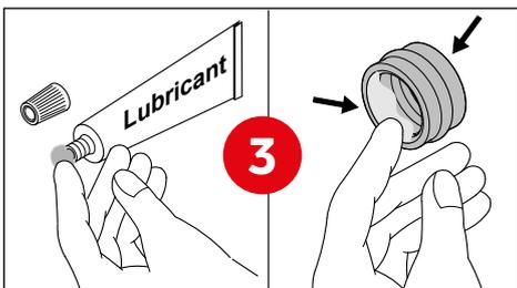
Lubricate and install the beater seal.
