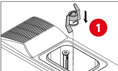
Place the hopper agitator on the specific housing.
