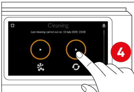
Activate the beater rotation and release the sanitizing solution.
