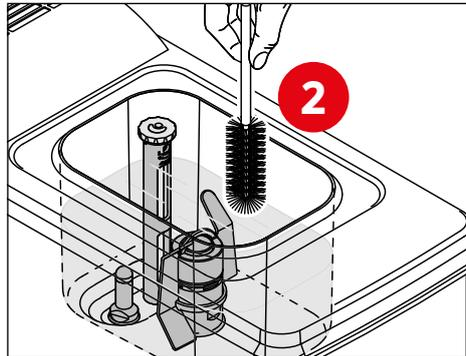
Brush the components, the hopper walls and the lower side of the hopper cover.
