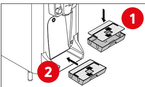
Fit the assembled drip-tray on its housing on the front panel.
