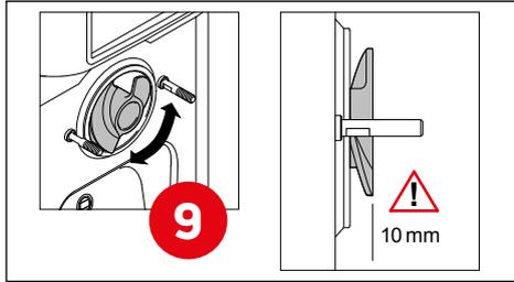
Insert the assembled beater in the freezing cylinder.
