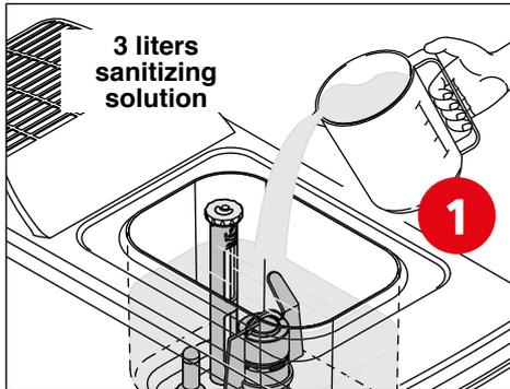
Prepare a sanitizing solution and pour 3 litres of sanitizing solution into the hopper.
