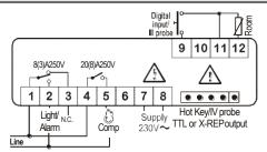
9-40Vdc supply: connect to the terminals 7 and 8. 12Vac/dc supply: connect to the terminals 7 and 8. 24Vac/dc supply: connect to the terminals 7 and 8. 120Vac supply: connect to the terminals 7 and 8.
