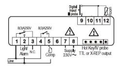
9-40Vdc supply: connect to the terminals 7 and 8.
